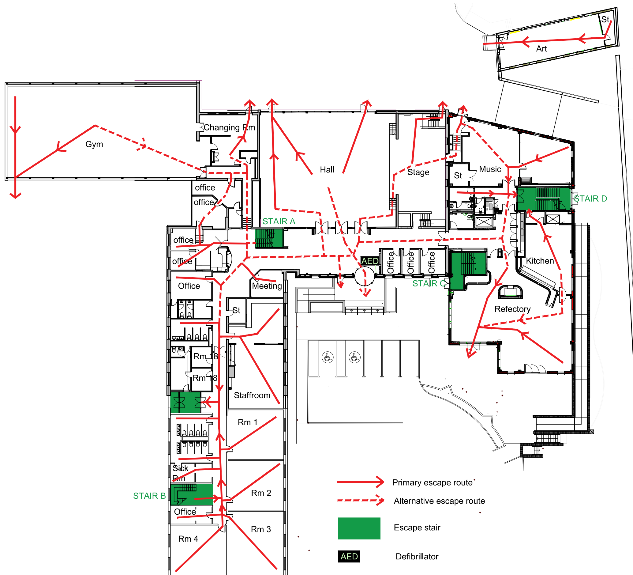
Ground floor emergency escape route plan.
